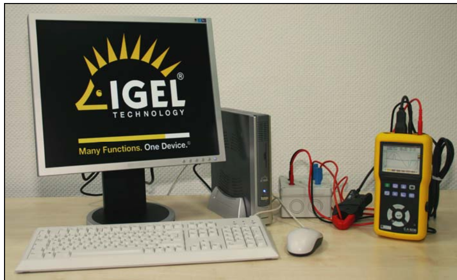
Figure 5-7: Measuring power on the IGEL Thin Client (Photo: Fraunhofer UMSICHT)
